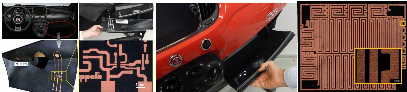
Fig. 2. Demonstrator of SSAIL: FIAT 500 gloves box touch-sensitive opening mechanism; circuit design for data protection.
